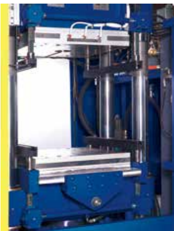
Top/ Bottom Hydraulic Mechanical Ejector, Synchronized Mechanism 上/下吊模裝置、同步機構
